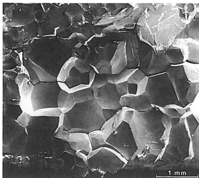
Figure 3: FEG-SEM fractograph at, and near, the external surface of a sample from the sawn-off slice. The fracture is almost entirely intergranular.
